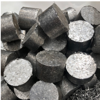
Briquettes produced from swarf
